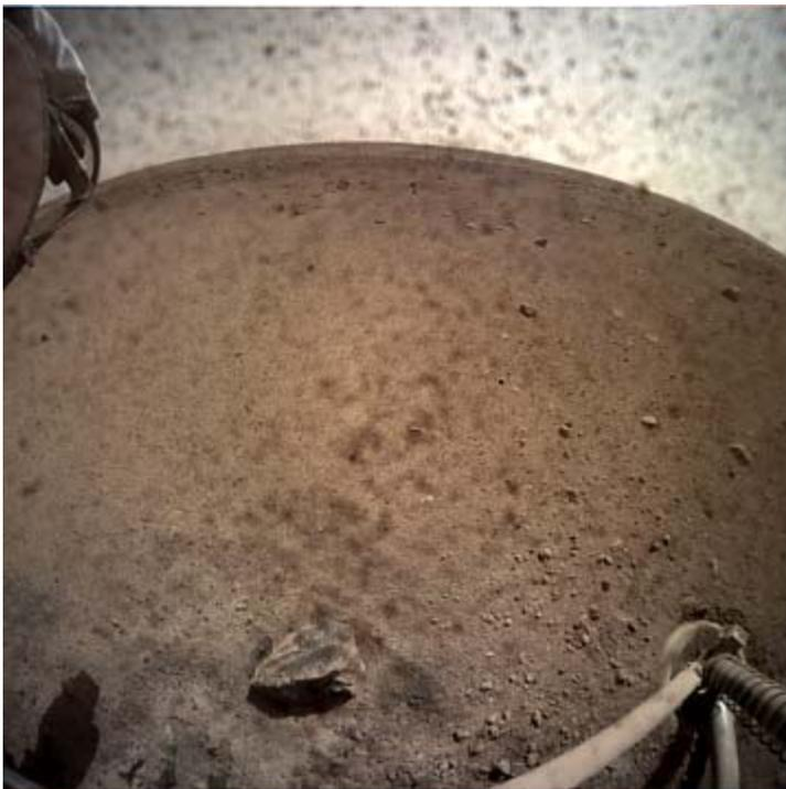
*Here is an image taken by the ICC after the dust cover was opened. The "port hole" appearance is now gone, but unfortunately it shows that some dust did get under the lens dust cover during the landing. The good news is that this image shows less dust than the one taken right after the dust cover was opened. It looks like the gentle Martian breezes are slowly removing the dust from the lens.*
