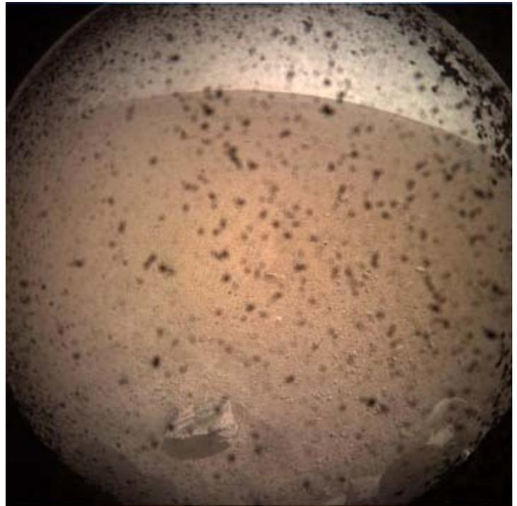
*The first image taken after landing using InSight's Instrument Context Camera (ICC). The camera's transparent dust cover was still in place when this image was taken. The cover is what makes the "through a port hole" appearance of this image. There is also a lot of dust, kicked up by the landing rockets, visible. Also visible in the image is a good sized rock, and one of InSight's legs and footpad in the lower right.*
