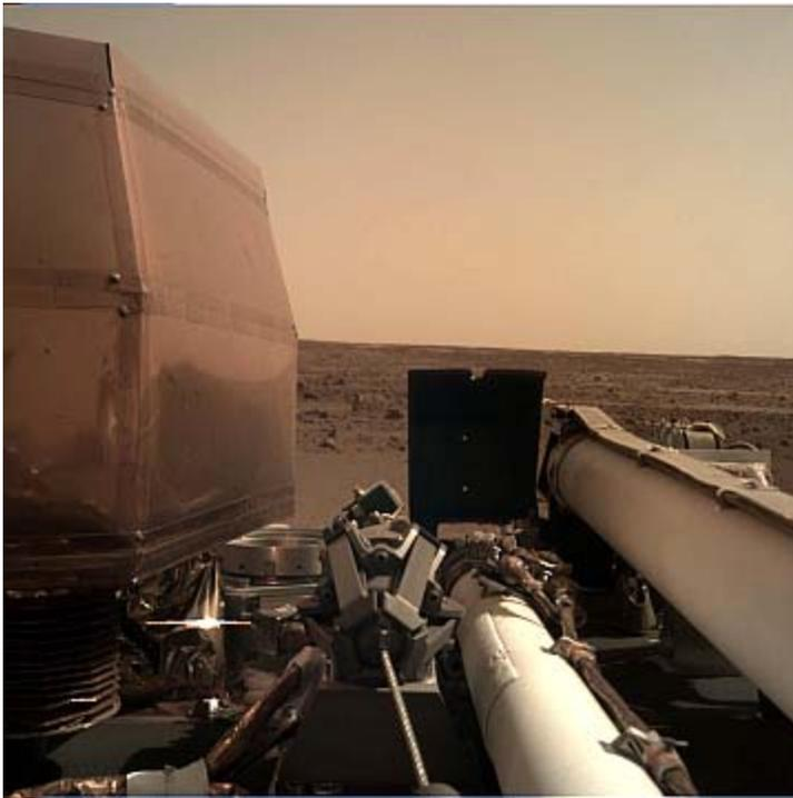
*This is the first image taken by the Instrument Deployment Camera (IDC), located on the robot arm on top of the spacecraft deck. This camera still has its dust cover in place, but there is almost no dust on it since its location on top of the deck protected from the dust blasted out by the descent engines. Part of the robot arm and the instrument grapple are visible in the center and right. The seismometer that will be deployed on the surface is the device on the left.*
