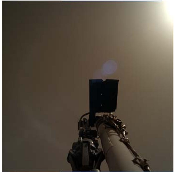
*This image taken by the IDC shows the robot arm partially deployed during its post-landing checkout. The sun is in the upper right.*
