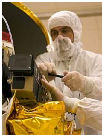
The Alice ultraviolet spectrometer aboard New Horizons. (Image: NASA/JHUAPL)
